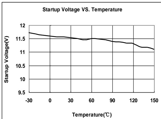
**(4) VDD under voltage lock out enter voltage vs. Temperature**
